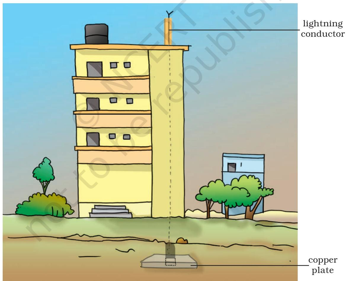
**Fig. 15.7 :** Lightning conductor
