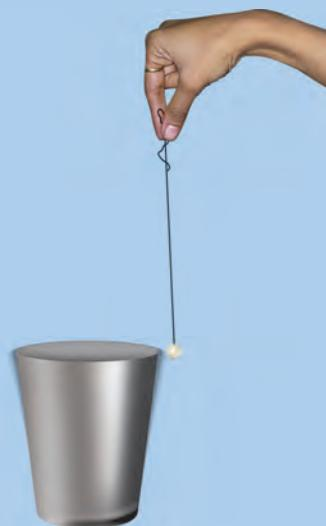
**Fig. 13.17 :** Thermocol ball touching the vibrating glass tumbler
