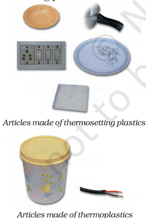
**Fig. 3.8** : Some articles made of plastic
