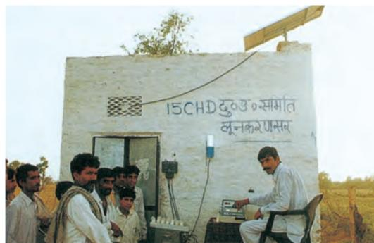
**Fig. 5.11:** Solar operated electronic milk testing equipment
