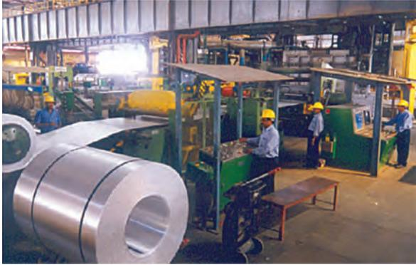
Fig. 6.6: Strip casting mill at smelter of NALCO
