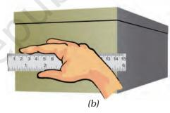
**Fig. 10.8** (a) Incorrect and (b) correct method of placing the scale with broken edge
