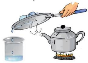
Fig. 5.13 Evaporation and condensation
