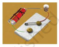
Fig 12.9 An electric circuit with a switch
