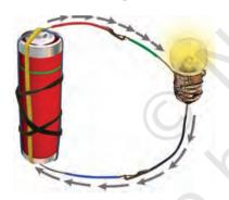
**Fig.12.6** Direction of current in an electric circuit
