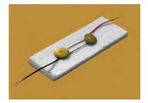
Fig. 12.10 A switch in 'on' position
