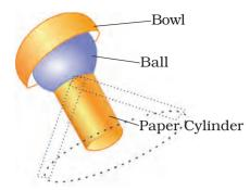
Fig. 8.2 Making a ball and socket joint
