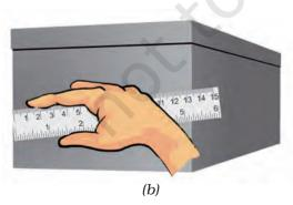
**Fig. 10.7** Method of placing the scale along the length to be measured (a) correct and (b) incorrect
