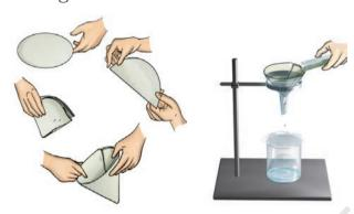
**Fig. 5.9** Folding a filter paper to make a cone
