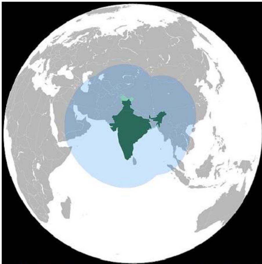
Figure 9: Illustration of the IRNSS coverage which includes an area of ~1500 km around the Indian landmass (image credit: ISRO)
